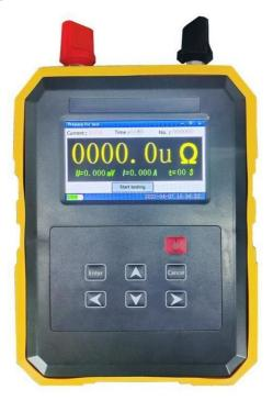
LCD screen: 4.3 inch industrial high brightness color LCD screen, display operation menu and display measurement results.
