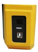
USB port: Connects to an external USB disk for storing test data.
