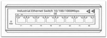
**Front panel:** The yellow light on the port is the LINK light, which is on when the connection is established and the data transmission is flashing. The green light is PoE light, which is only on when the switch port is supplying power to the PD devices. Power indicator light is on when connecting with Power.
