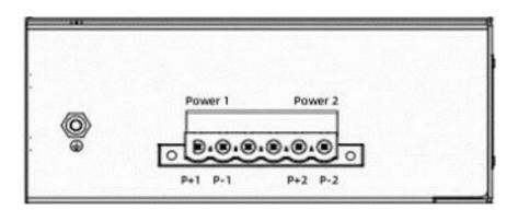
**Side panel:** P1 and P2 are the number of connecting terminals, P+1 and P-1 are respectively to the positive and negative poles to be connected; Earthing screw, used for earthing equipment.
