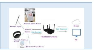
BLE Scan Gateway Automatically Scan Bluetooth Device via Bluetooth, Upload Data to PC / Server
