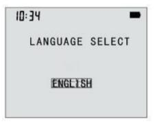
After entering the menu, short press the left button or right button to select the "Language" option, short press the middle button to enter the language selection interface, press the left button or right button to select the type of prediction, confirm the long press the middle button to exit the language selection interface, return to the menu interface.
