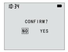
After entering menu, short press the left button or right button to select the "Factory Reset" option, short press the middle button, the instrument restores the factory set.
