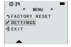
After entering the settings interface, short press the left button or right button to select the "Exit" option, short press the middle button, the screen will automatically exit the settings interface and return to the previous menu.
