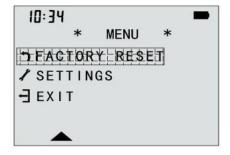
Press and hold the middle button to enter the shutdown interface. At this time, press the middle button twice to enter the user menu interface.
