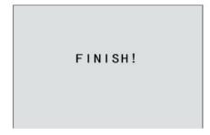
After entering the menu, short press the left button or right button to select the "SELF TEST" option, short press the middle button, it enters the self-test state. The display shows red, yellow, blue, white and black in turn, the lights flash in sequence, and the buzzer sounds once. It loops twice like that. After the self-test is completed, the display shows "Finish" and then enters the display concentration interface.
