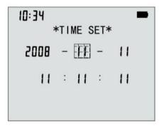
After entering the menu, short press the left button or right button to select the "TIME SET" option, short press the middle button to enter the time setting interface. Short press the middle button to select the time option you want to modify, press the left button or right button to modify the option content. After the modification is completed, long-press the middle button to exit the time set option and return to the menu interface.
