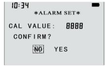
middle key to enter. In the setting, short press the left or right button to adjust the value, and short press the middle button to adjust the number of digits. After the modification is completed, long press the middle button to jump to whether to confirm, short press the left button or the right button to select "Yes" or "No", and return to the factory setting interface after confirming.
