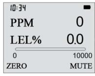
preheating is completed, it enters the zero point compensationIf the interface is in fresh air, select "Yes", and then enter the main interface, which can be used normally.
