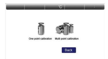
When the instrument error or improper operate. Calibration weights can be adjusted with accuracy.Press "One point calibration" and does not release until it display "-cal-",Then flashing put on the "100.000", put on the calibration weight, then it will display "= = = = = =", until it display "100.000",and will show remove the weight, it will display "= = = = = "again, Waiting it show" 0.000 ", the calibration is completed.
