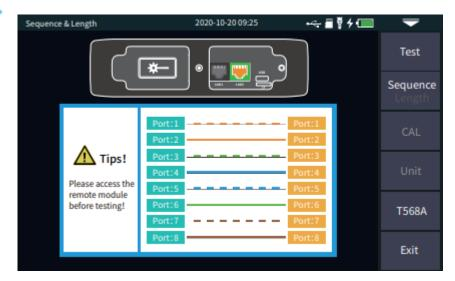
Direct connection test: during the test, the indicator lights of the host and remote device flash from 1 to 8 one by one.
