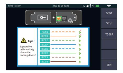
Test: turn on RJ45 cable tracking function. The line finding mode of this machine is digital radar type, which has strong anti-jamming ability. According to the target distance and proximity, the frequency of prompt tone is different.
