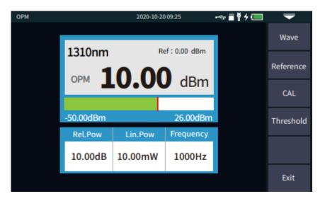
The conversion relations of absolute power, relative power and linear power are as follows: PAbs.Pow=10lgPLin.Pow/1mW
