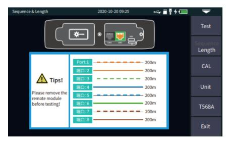
Cable length test: test the length of network cable.
