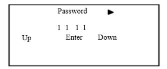
After entering the correct password by pressing the button, enter the menu selection. If the password is wrong, it will return to the gas display main page with a voice "password error" prompt.
