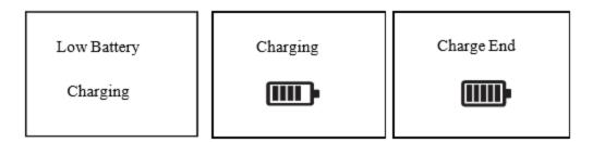
When the battery is less than 1 grid, the detector will automatically shut down to prevent data loss inside the detector and unpredictable damage caused by insufficient voltage on the internal sensitive components of the instrument.
